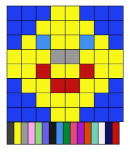
The corresponding array of color IDs is the same size and represents the same image, except that each color is replaced by its palette ID (0x00 to 0x0F):
