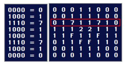
The SNES 4bpp format is not made to be human-readable, and it was made this way because of the hardware. Don't worry if you struggle with this; this is the detailed technical side and mastering it is not required at all to sprite. Same goes for the coming palette description.
